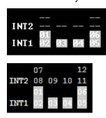
In an internal array of hot-swappable disks, the disks are numbered as follows from 1 to 6 or 12:
