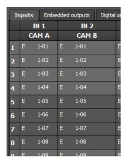
You will allocate the source audio mono channels as shown above when you want to send the audio mono channels from REC1 to all other record channels.
