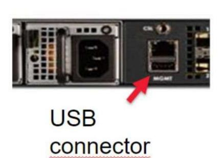
Once the USB key is plugged into the XHub. Please go to the front of the XHub and press the reset button for 4 seconds.
