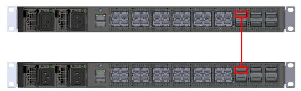
In most cases, a single uplink is realized between two XHub-VIA switches. See section "Single Uplink" on page 20.
