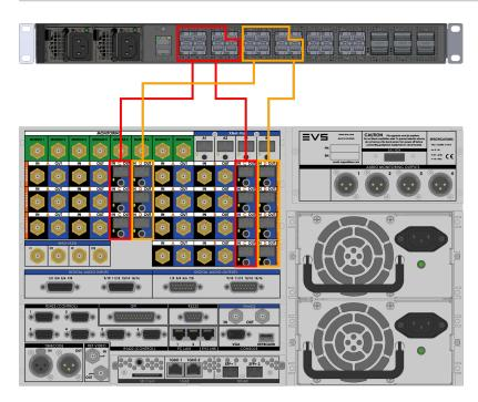
The ports 17-24 on the XHub-VIA switch are not active.
