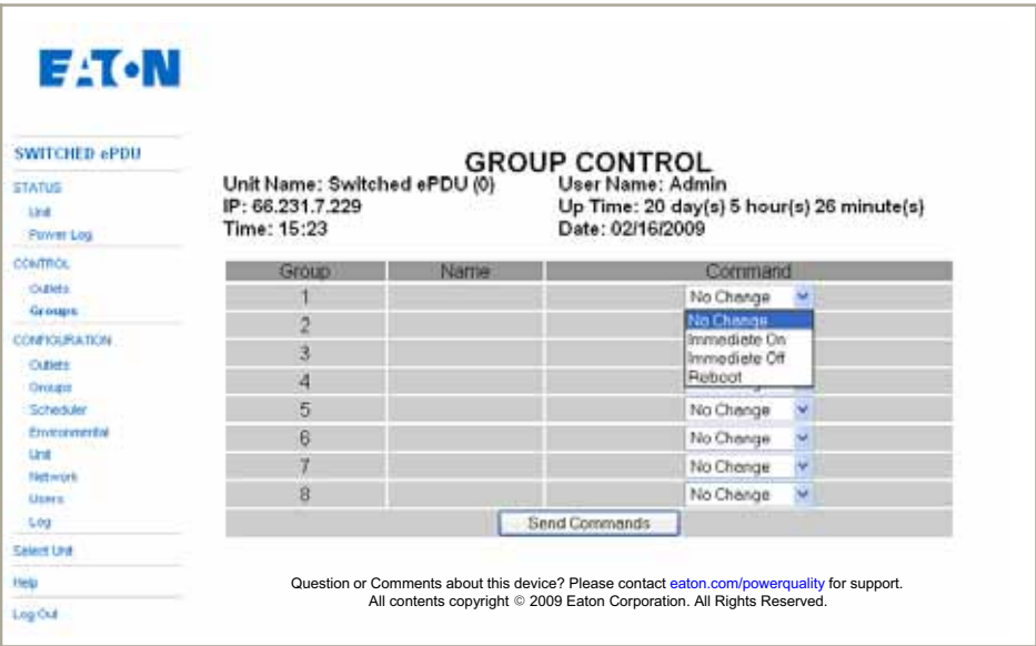
Figure 18. Group Control Page (Typical)
