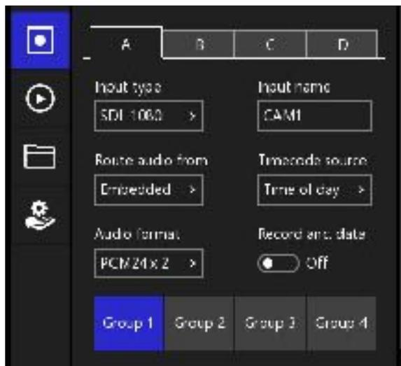
Each group is 4 channels of embedded audio. Each video input allows for up to 8 channels.
