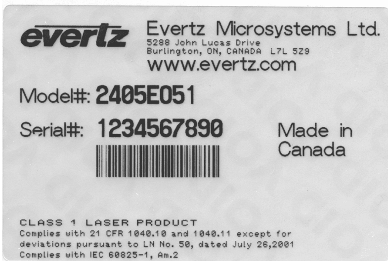
Typical 2405EO Certification and Identification Label (Serial # and bar code differ from unit to unit)
