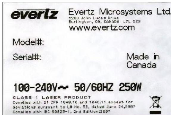
**Figure 2-6: Reproduction of Laser Certification and Identification Label**
