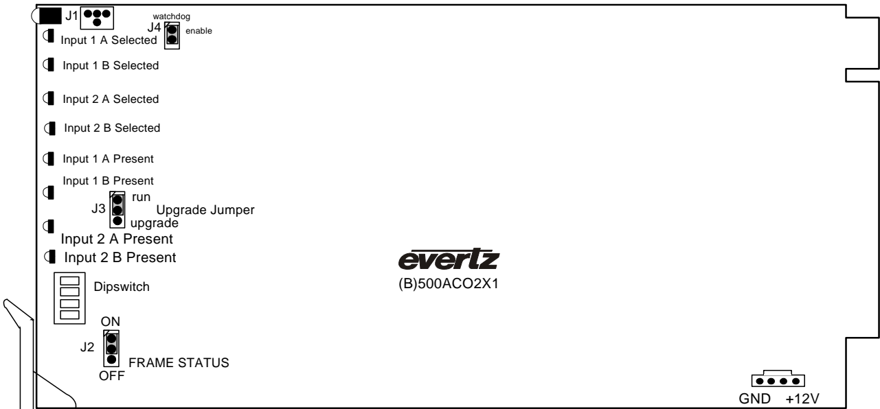
Figure 6-1: LED and Jumper Locations
