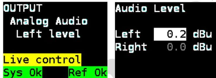
Figure 3-5: Adjustment Live Control
