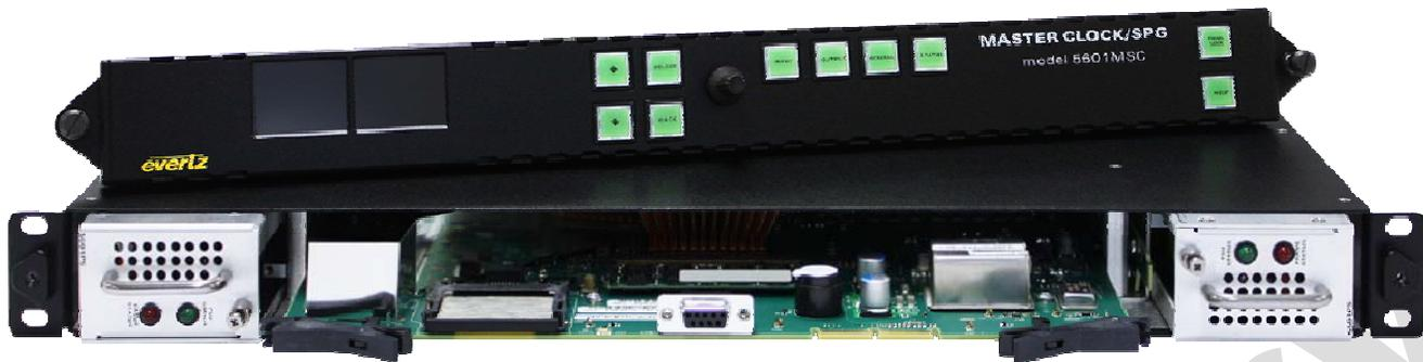
Figure 1-3: 5601MSC with Front Panel Removed and Other Components Partially Extracted
