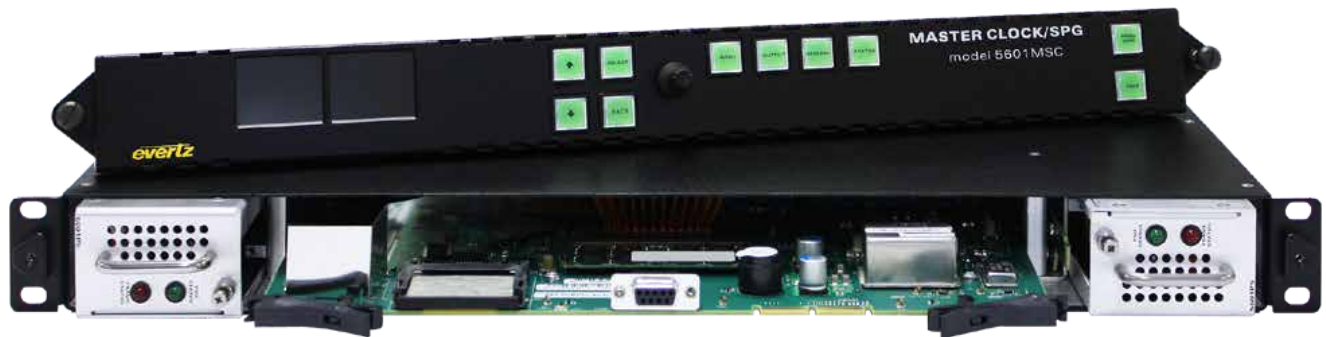
Figure 1-2: 5601MSC with Front Panel Removed and Other Components Partially Extracted
