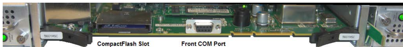
Figure 1-4: Front Panel Removed, CompactFlash Location
