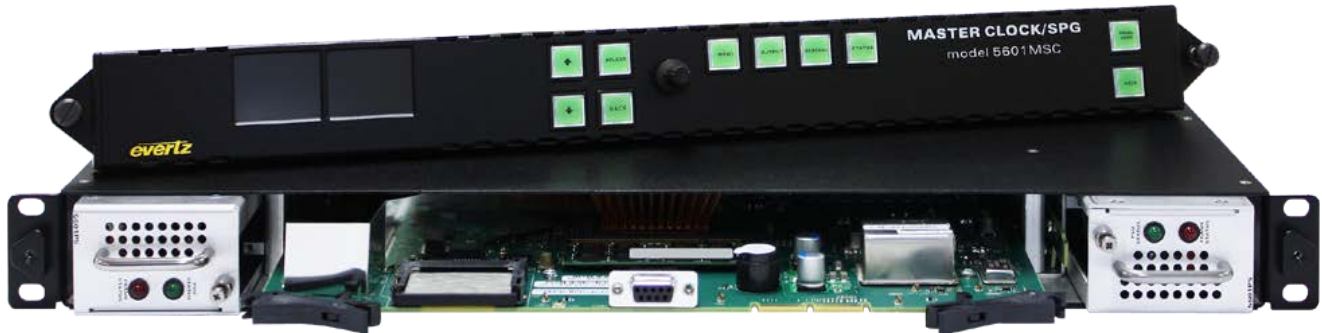
Figure 1-2: 5601MSC with Front Panel Removed and Other Components Partially Extracted
