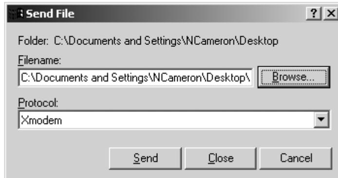
If you do not start the upload within 10 minutes the Boot code will time out. You can restart the upgrade process by removing and reinstalling the module.
