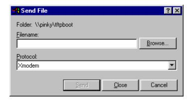
The "Folder" header describes the folder location of the previously downloaded Upgrade Program. To change the location/name of the file, use the "Browse..." button to locate and select the correct file. Make sure the Protocol is set to "Xmodem" and press the "Send" button to send the file.
