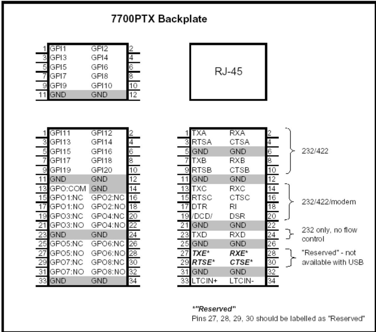
**Figure 3-2: Back Plate Connections**
