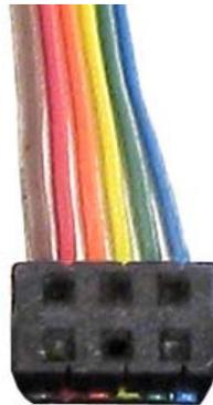
2. Connect it to the four-pin interface (J1) near the front of the 7700PTX, directly above the card unlock latch.
