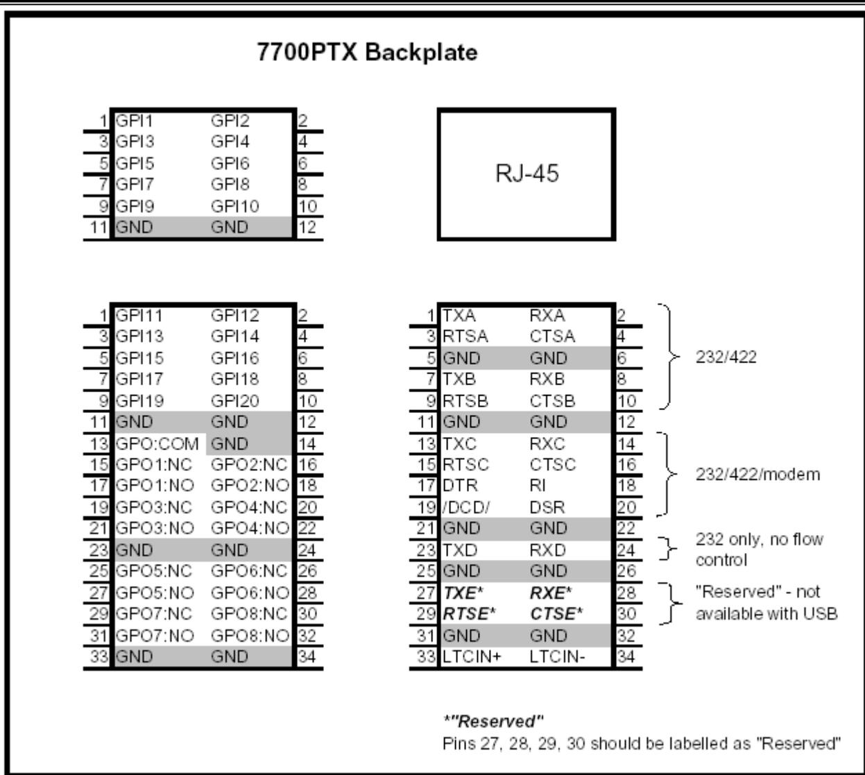
**Figure 2-2: Back Plate Connections**
