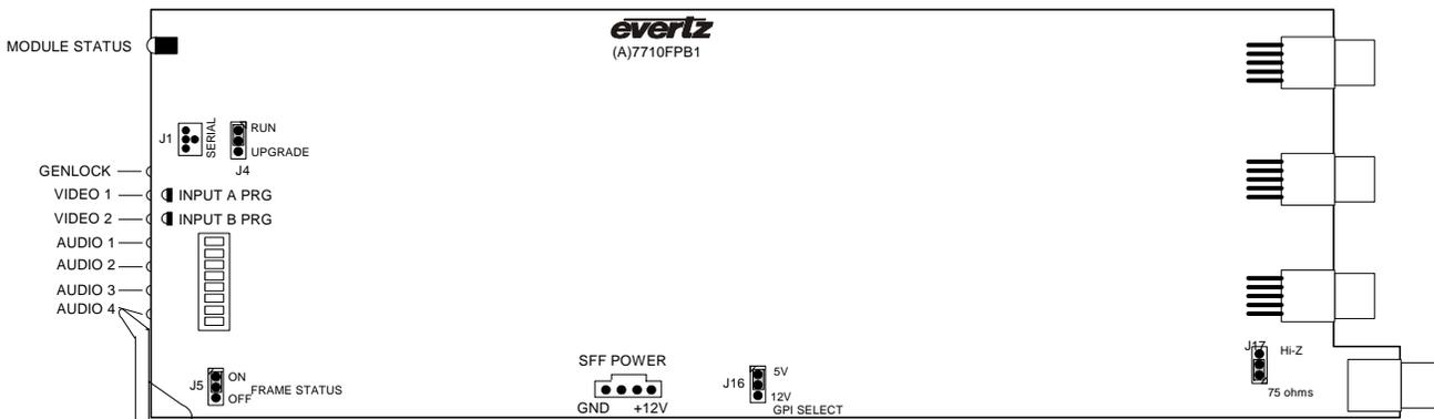
Figure 7-2: LED and Jumper Locations on REV A Boards
