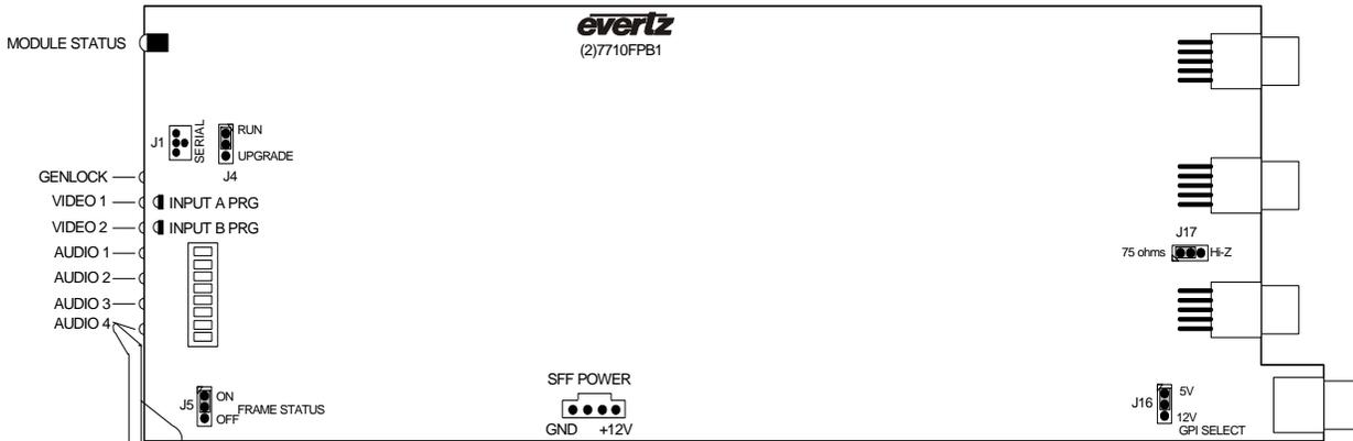
Figure 7-1: LED and Jumper Locations on REV 2 Boards
