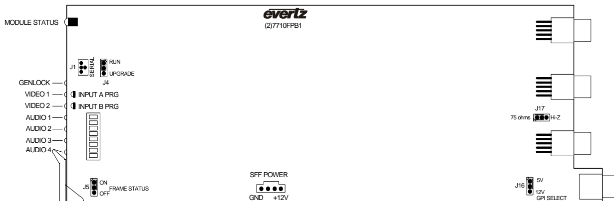
Figure 8-1: LED and Jumper Locations on REV 2 Boards
