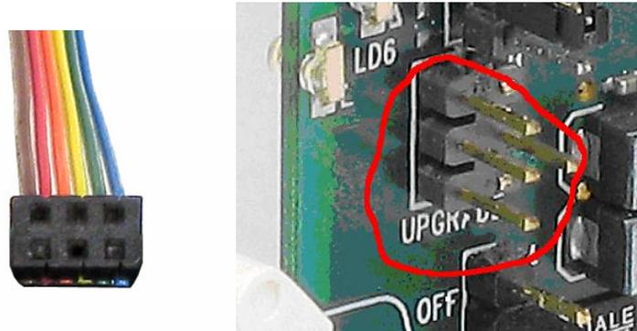
**Figure 4-1: Upgrade Cable and PCB Connector for Serial Connection.**
