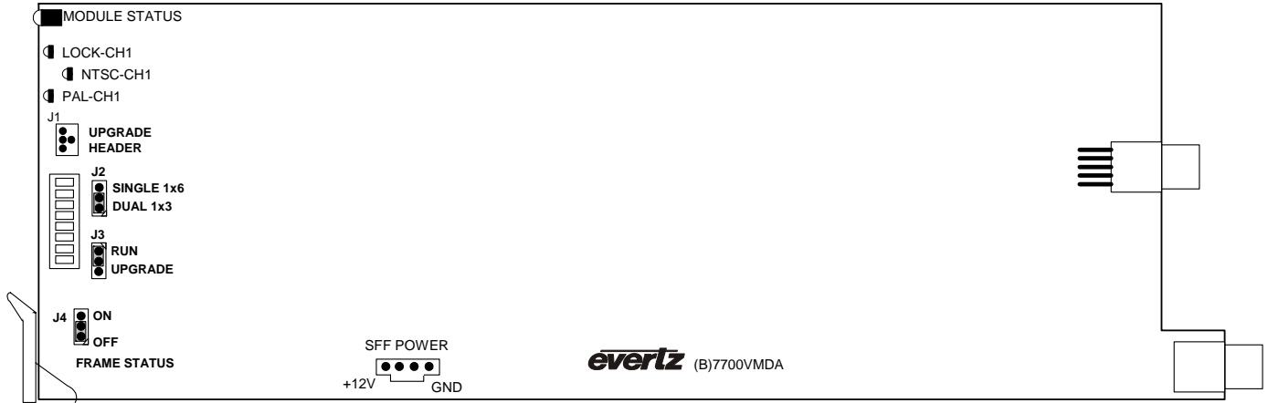
Figure 8: LED and Jumper Locations (Rev B)
