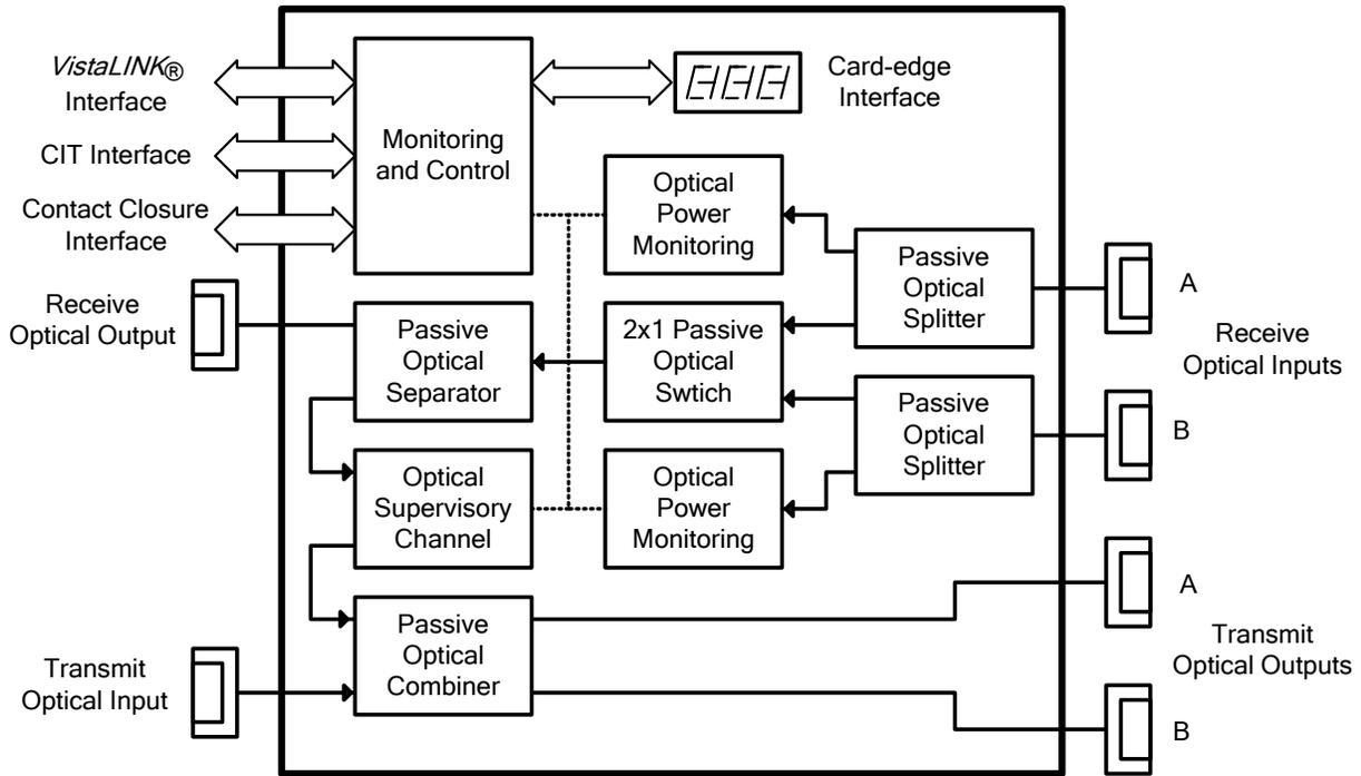
Figure 1-1: 7707BPX-TR Block Diagram
