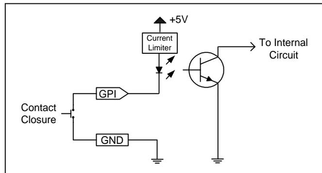
**Figure 2-2: Contact Closure Input Circuitry**
