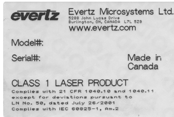
Figure 2-2: Reproduction of Laser Certification and Identification Label
