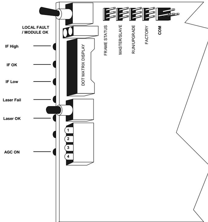
Figure 6-1: Location of 7707IFTA Jumpers and LEDs
