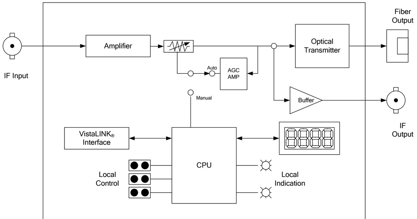
Figure 1-1: 7707IFTA Block Diagram
