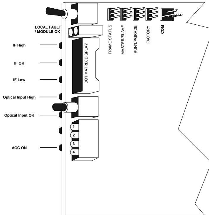
Figure 6-2: Location of 7707IFRA Jumpers and LEDs
