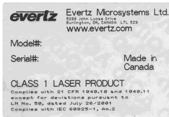
Figure 2-3: Reproduction of 7707LTA Certification and Identification Label for Models that are Class 1 Laser Products
