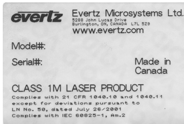
Figure 2-4: Reproduction of 7707LTA Certification and Identification Label for Models that are Class 1M Laser Products
