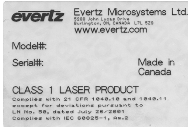
Figure 2-2: Reproduction of Laser Certification and Identification Label
