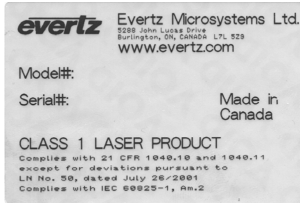
Figure 3: Reproduction of Laser Certification and Identification Label
