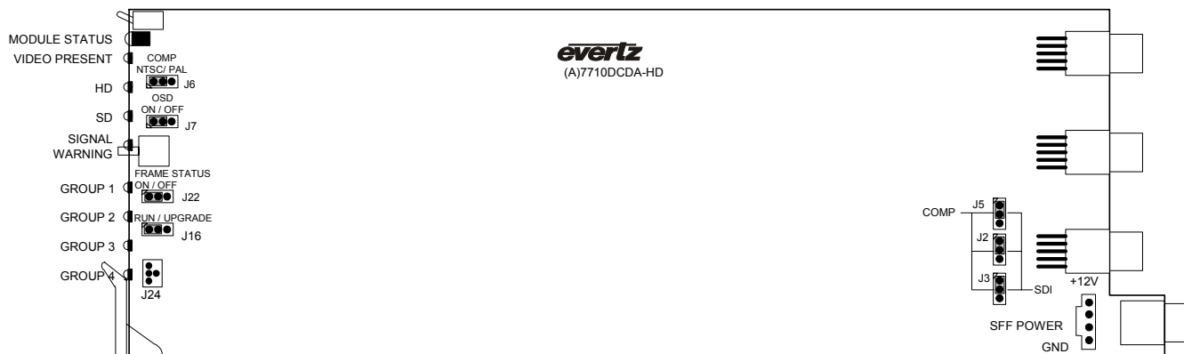
Figure 6: LED and Jumper Locations – Rev A Boards
