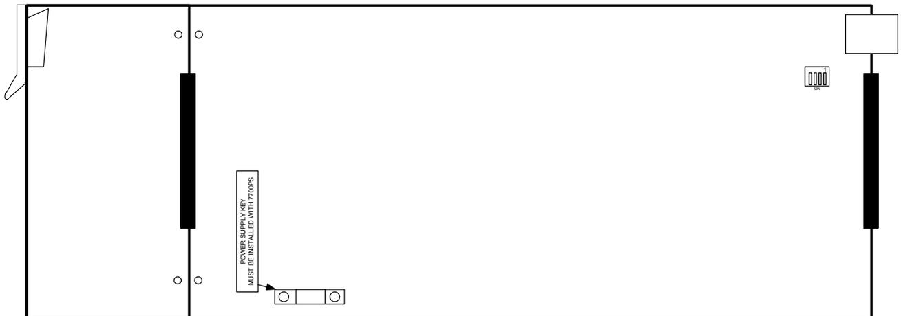
Figure 6-2: Location of Jumpers – Bottom View Main Module
