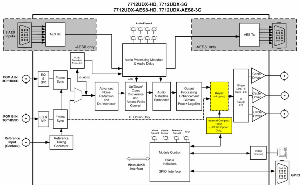
**Figure 1-1: 7712UDX Block Diagram (-HD, -3G and –AES8 Versions)**
