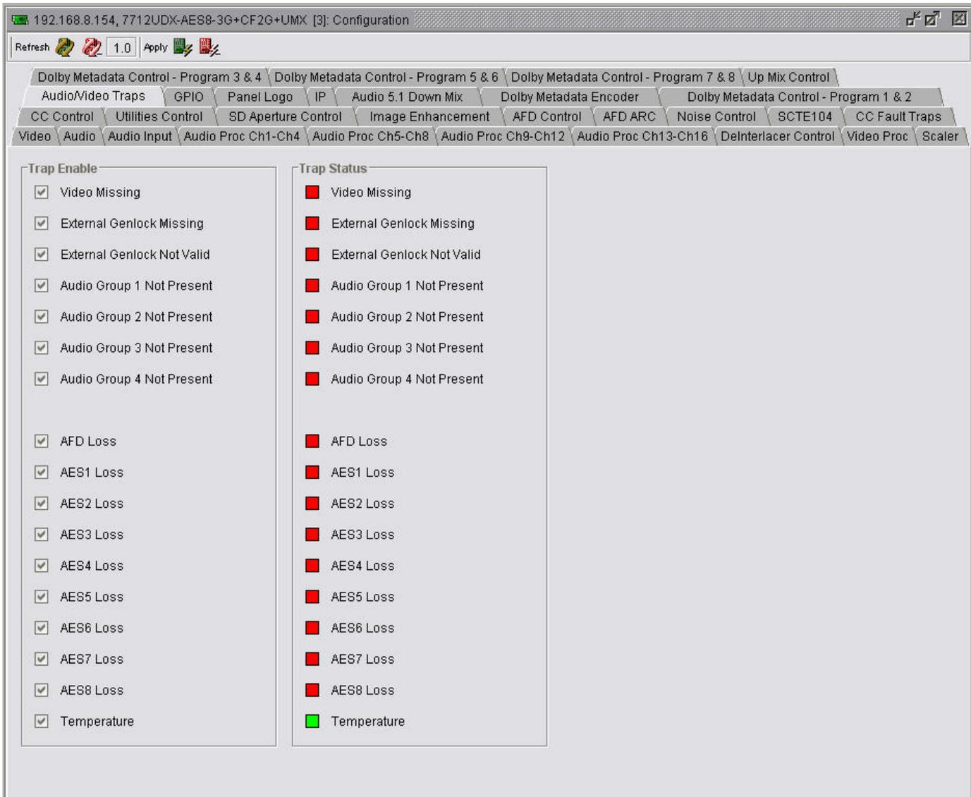
Figure 5-17: Audio/Video Traps Tab
