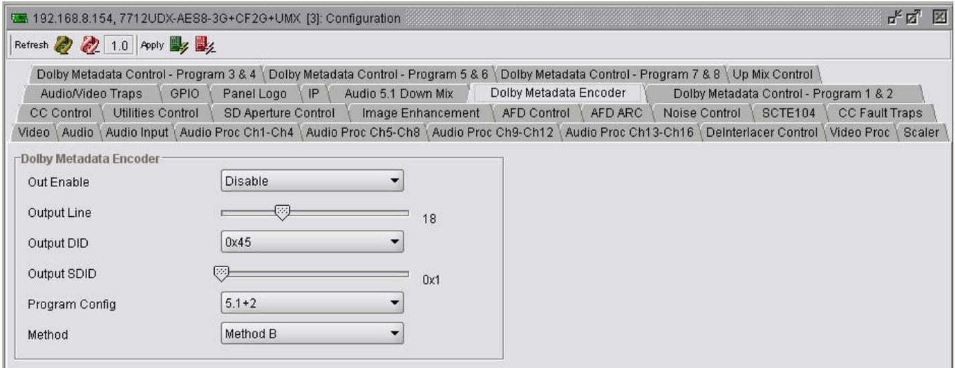
Figure 5-22: Dolby Metadata Encoder Tab
