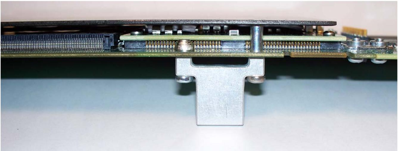
**Figure 6-3:Slot Blocker Installed**
