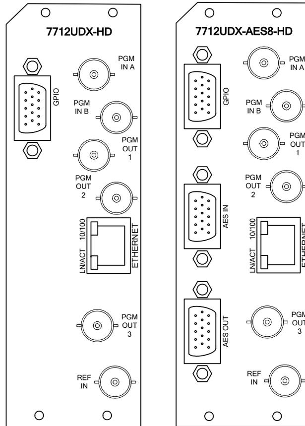
Figure 2-1: 7712UDX-HD & 7712UDX-AES8-HD Rear Panels
