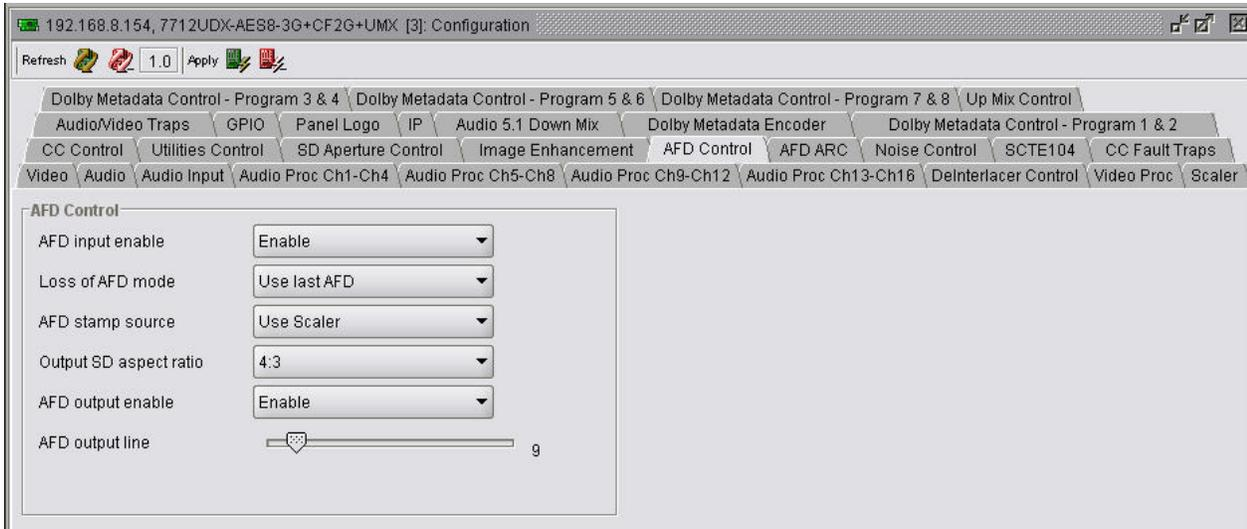
Figure 5-12: AFD Control Tab
