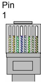
**Figure 2-3: Colour Code Wiring for the Current RJ 45 Standards**
