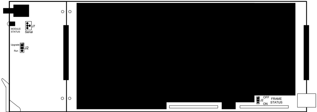
Figure 6-1: Location of Jumpers – Top View Main Module
