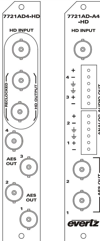
Figure 2: 7721AD-HD Series Rear Panels
