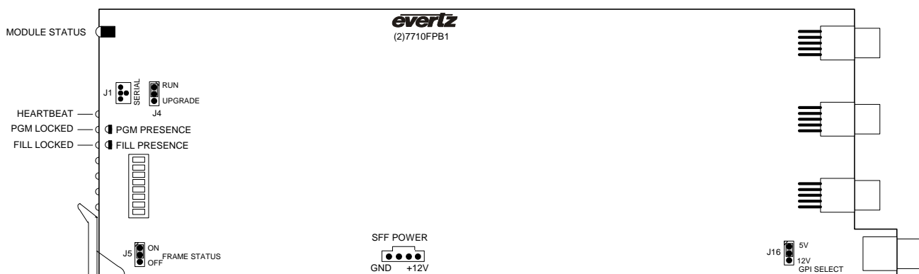
Figure 6-1: Location of Jumpers on Main Board (Rev. 2)
