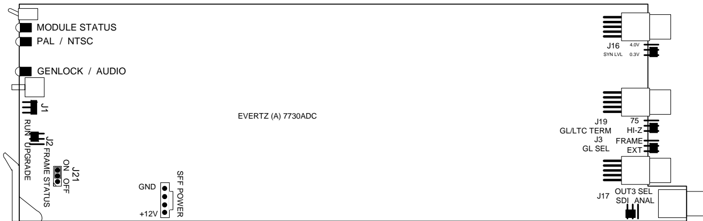
Figure 10-1 : Location of Jumpers on 7730ADC Main Board
