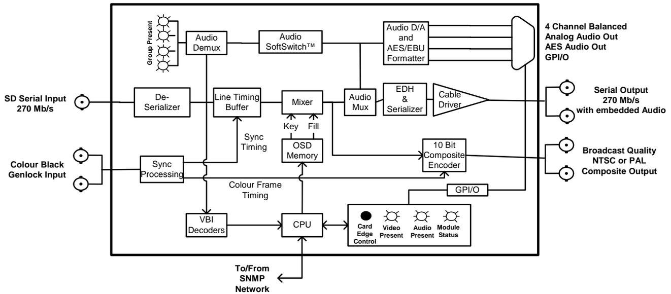
**Figure 1-1: 7735AVC-LB Block Diagram**
