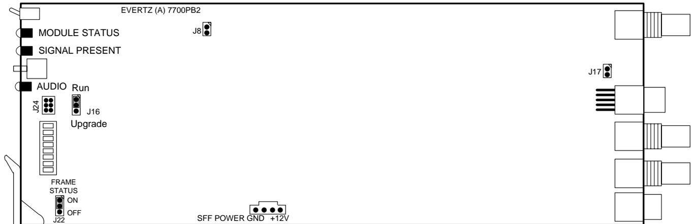
Figure 10-1: Location of Jumpers on 7700PB2 Boards
