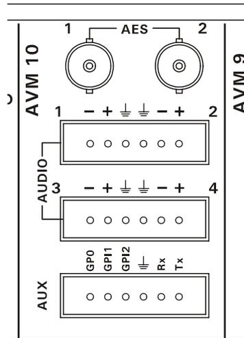
**Figure 2-4: Breakout Panel for Wiring Audio and Aux Connections**
