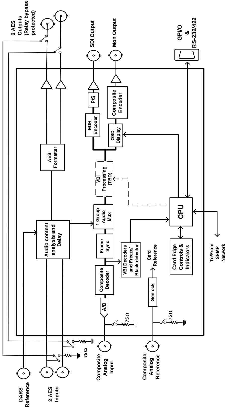
Figure 1-2: 77CDM-AES Block Diagram
