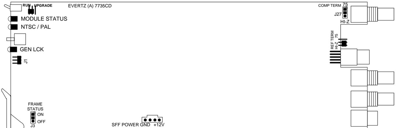
Figure 9-1 : Location of Jumpers on 7735CD Main Board
