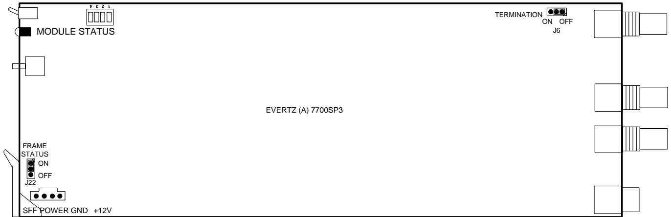
Figure 8-1: Location of Jumpers on Main Boards
