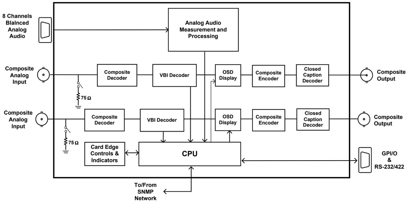
Figure 1: 7761AVM-DC Block Diagram
