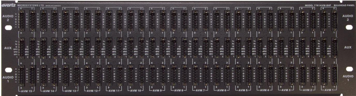
A 7761AVM-BHP bulkhead breakout panel is available to facilitate wiring to the DB-25 connector. This panel allows for convenient audio, GPI/O and RS-232 connections for up to 15 7761AVM-DC cards 3 RU panel.
