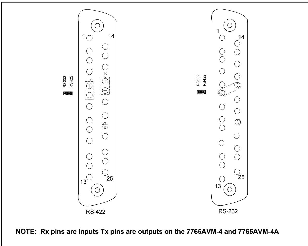
**Figure 5: AUDIO AND AUX I/O Physical Layout and RS-232/422 Serial I/O Pin Connections**
