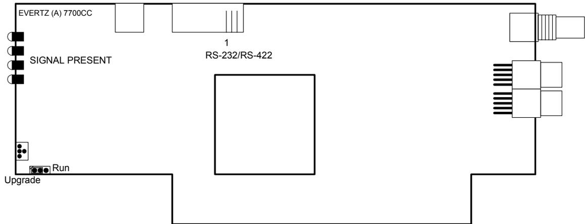
Figure 7: Location of Jumpers on 7700CC Boards
