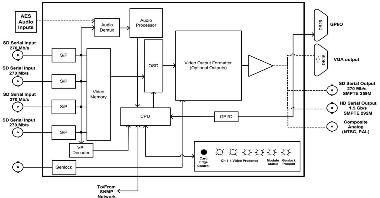
**Figure 1: 7765AVM-4 and 7765AVM-4A Block Diagram**
