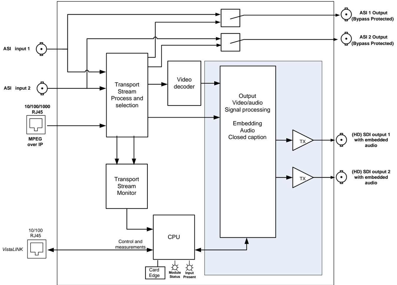
Figure 1-1: 7780DEC-MP2HD Block Diagram
