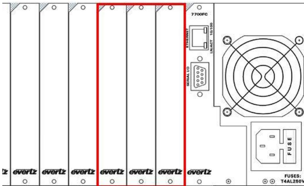
Figure 2-2: 7700 Chassis and 7780DEC-MP2HD Rear Panel
