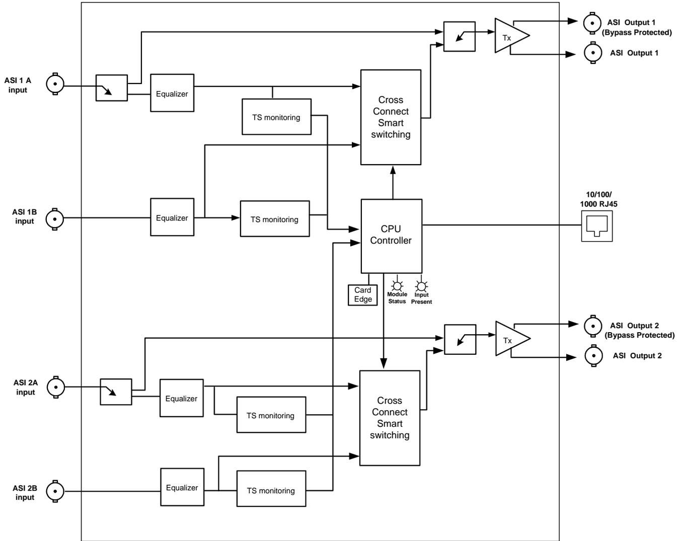
**Figure 1-1: 7780R2X1-CS-2 Block Diagram**
