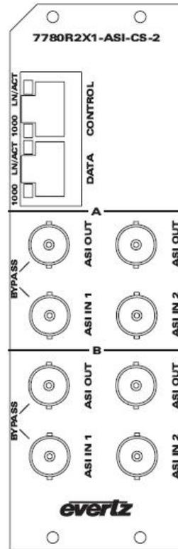
**ETHERNET:** The upper Ethernet port is for VLPro control and should be connected to the control network. Connection should only be made to the network once the initial IP configuration has been completed.
