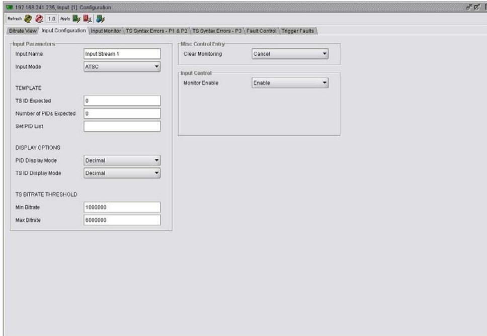
Figure 4-2: VistaLINK® PRO Input Configuration Tab
