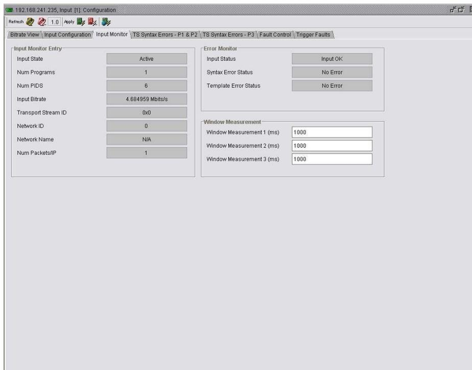
**Figure 4-3: VistaLINK® PRO Input Monitor Tab**
