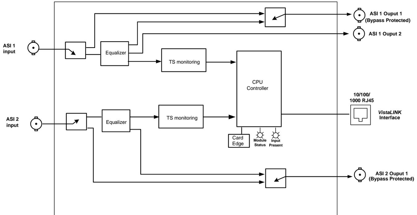
Figure 1-1: 7780TSM-ASI Block Diagram
