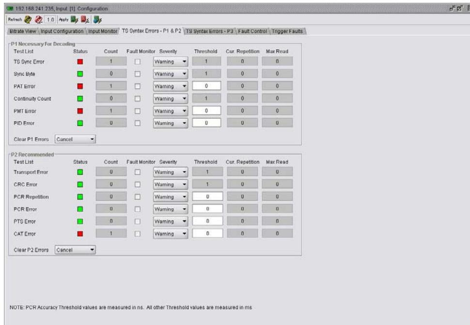
Figure 4-4: VistaLINK® PRO TS Syntax Errors – P1 & P2 Tab
