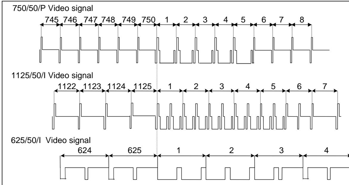
**Figure 3-4: Default Signal Alignment in 50 Hz Field Rate Systems**
