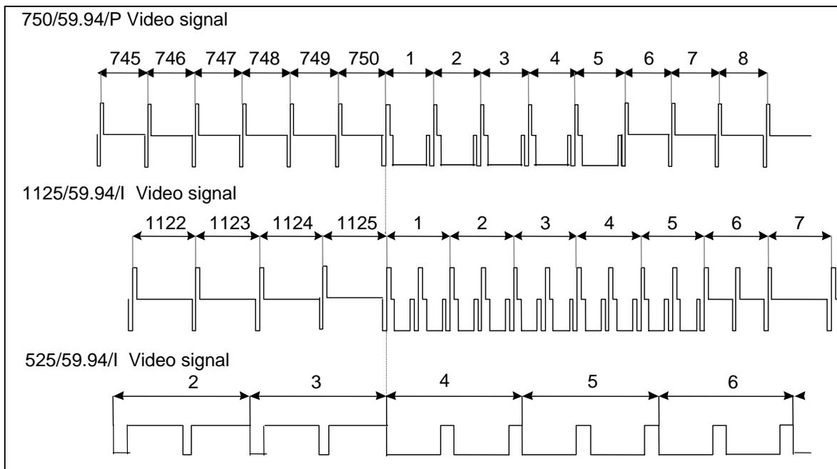
**Figure 3-3: Default Signal Alignment in 59.94 Hz Field Rate Systems**
