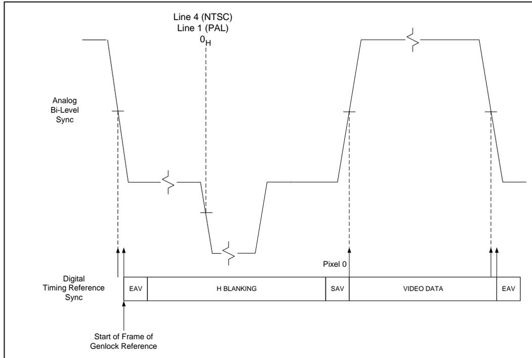
**Figure 3-2: Default Bi-Level Genlock Reference Timing**
