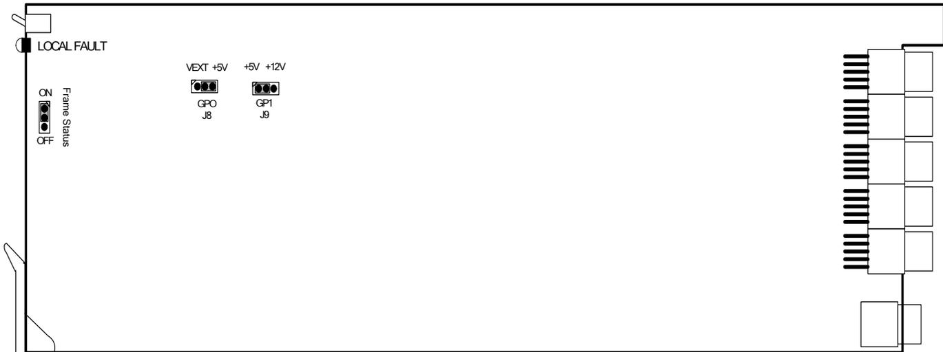
Figure 6-3: Location of Jumpers Bottom Board (A7700 G4-AUX-IO)
