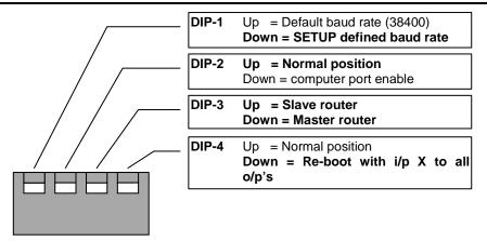
The normal setting for a master router is Up,Down,Down,Up and for a slave router Up,Down,Up,Up.
