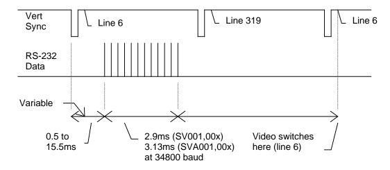
The delay between the vertical sync and the RS232 message can be adjusted from 0.5ms to 12ms and this has no effect on the video switch point. Delays between 12ms and 18ms cause the video to start switching in this frame OR the next frame some of the time. A delay beyond 19ms causes the video always to switch in the next frame.
