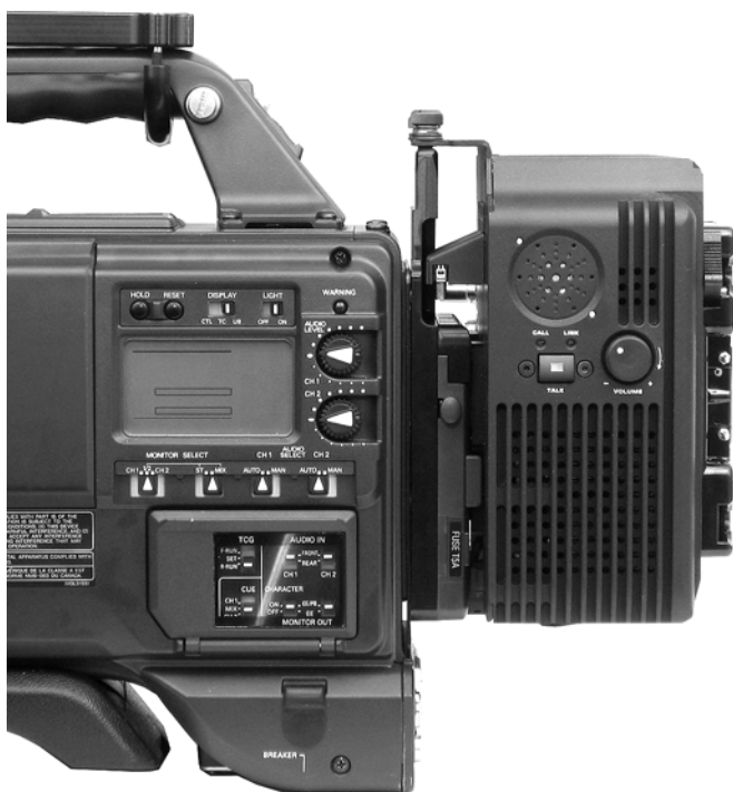
Figure 2-5: ECAS-HD Mounted on Rear of the Panasonic Camera using Mounting Kit Adapter Plate
