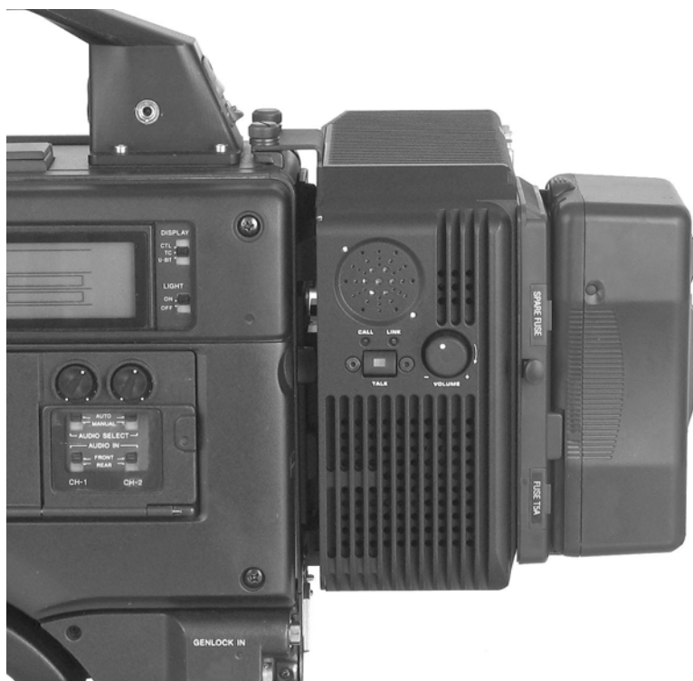
Figure 2-2: ECAS-HD Mounted with Battery Pack
