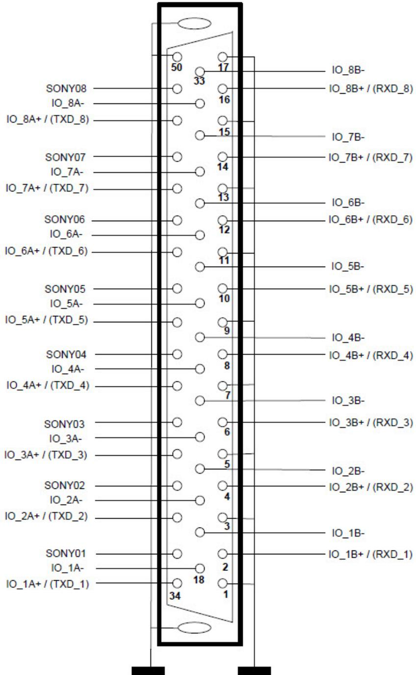
**Figure 2-26: Data Port Pin-Out**
