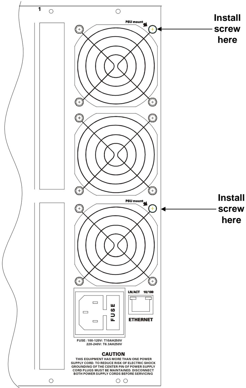
**Figure 2-28: Locating the Power Supply Mounting Screw**
