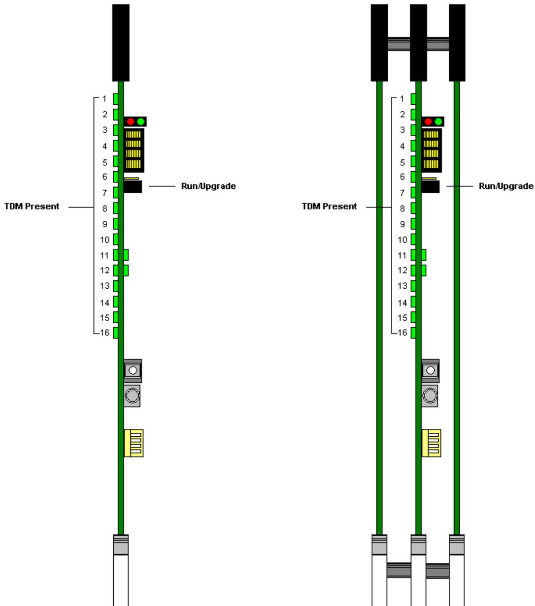
Figure 2-16: EMR-ADMX-16X16 (left) and 3000ADMX-16X16 (right) Front Card Edges
