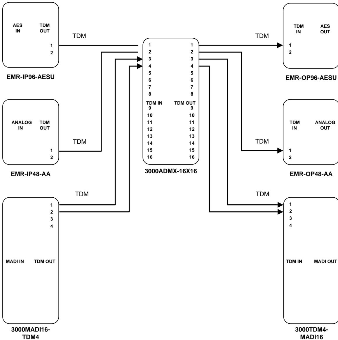
**Figure 4-2: EMR Audio Connected with TDM Interface**
