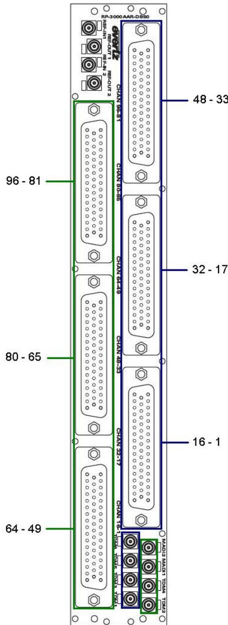
Figure 2-11: EMR-IP48-AA Rear Plate Connection Details (MADI Firmware)
