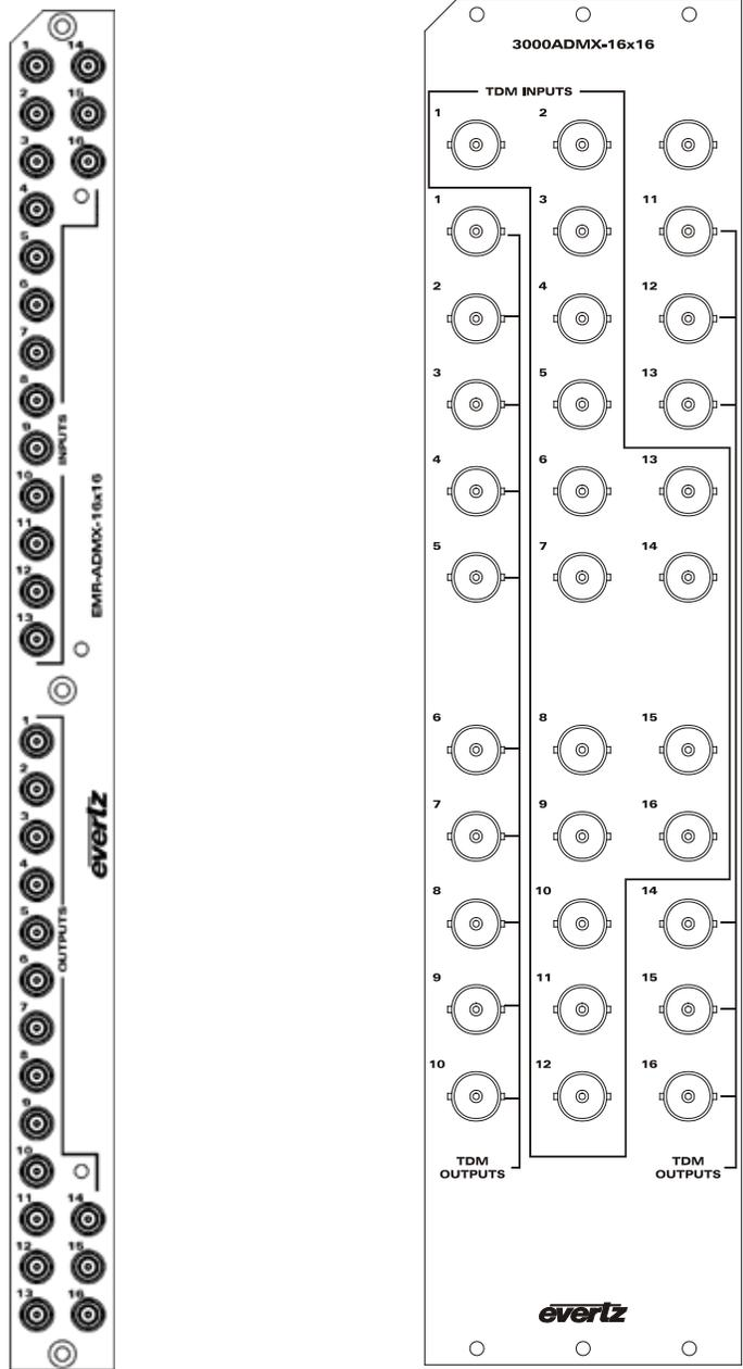
Figure 2-15: EMR-ADMX-16X16 (left) and 3000ADMX-16X16 (right) Rear Plates
