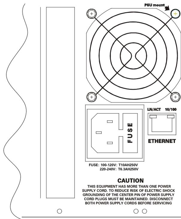
Figure 2-29: Connecting the Power to the Frame
