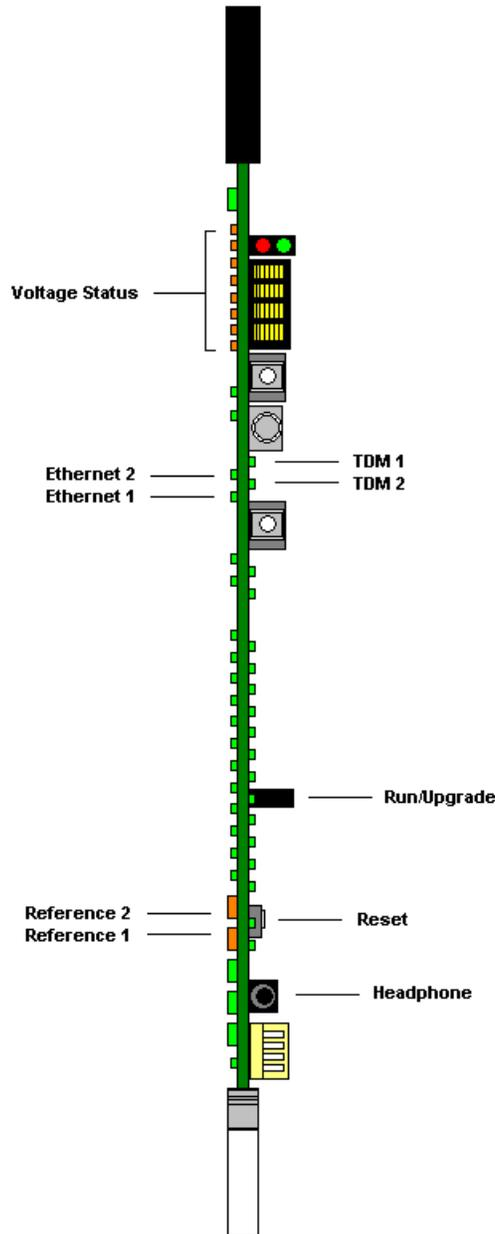
Figure 2-27: EMR-PR48 Front Card Edge
