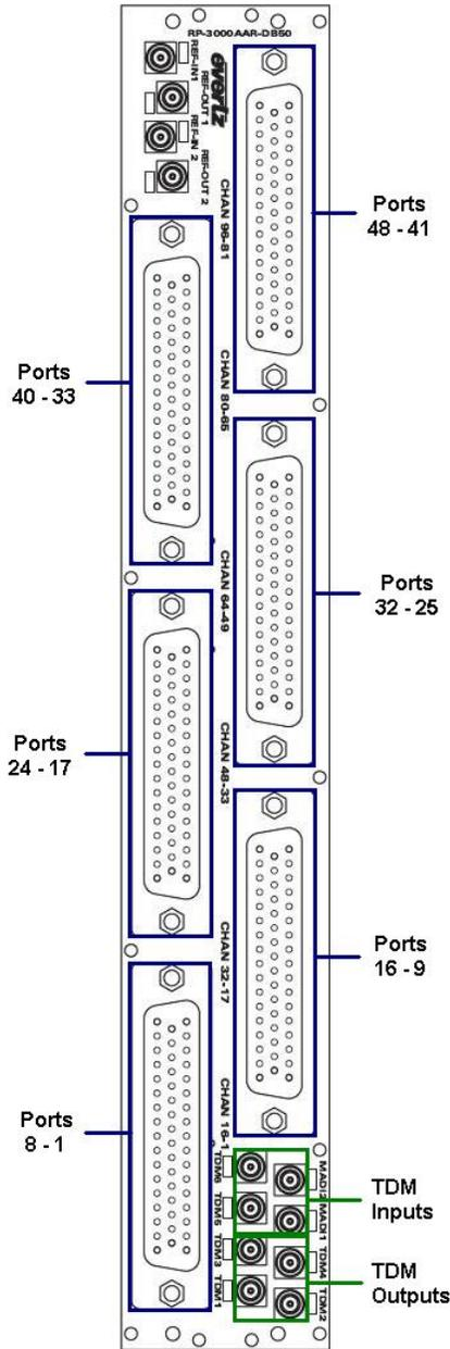
**Figure 2-25: EMR-PR48 Rear Plate**
