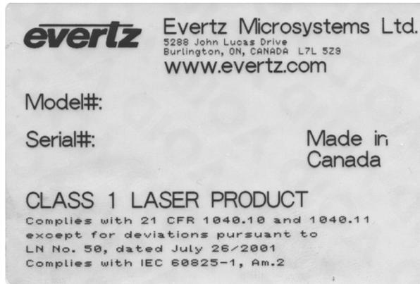
**Figure 2-31: Reproduction of Laser Certification and Identification Label**
