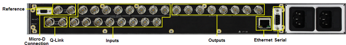
Figure 4-3: Rear Communication Connections on EQT-1602-CS Newer Rear Plates
