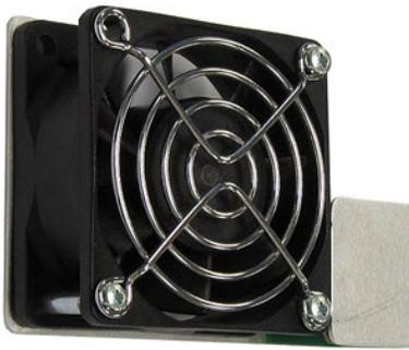
Each of the crosspoint fan modules can be simply and quickly removed and replaced while the crosspoint module is still in place and operational.
