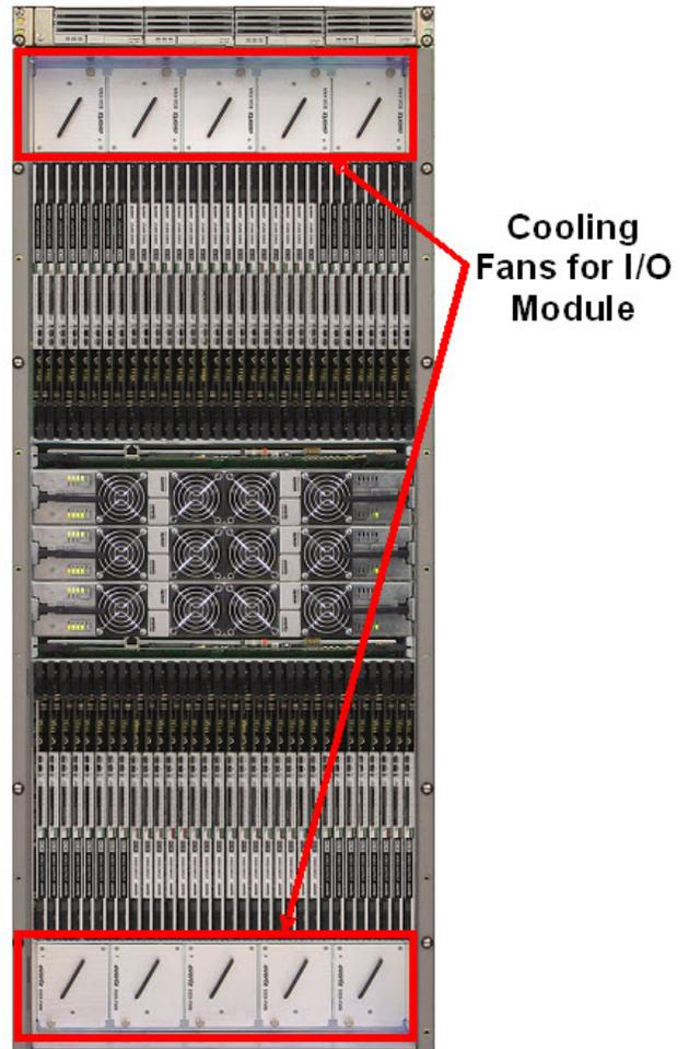
The air-flow through the EQX is from front to rear. The cool air enters the frame at the front, passes over the input and output modules and then exits through the rear of the frame.
