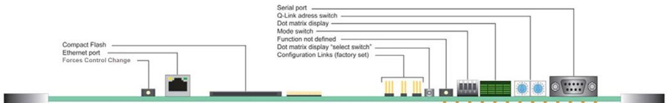
Figure 5-1: Frame Controller Module Card Edge Controls and Connectors
