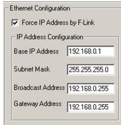
**Figure 8-4: Ethernet Configuration Window**
