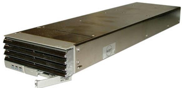
The external power supply for the EQX is a single rail, load-sharing design. It is housed within a single 1RU rack-mounting tray (EQX-PS-FR), which carries four power supply modules (EQX-PS), each with their own AC inlet. Power supply modules operate on either 100-115 or 220-240 volts AC at 50 or 60 Hz and automatically sense the input voltage.
