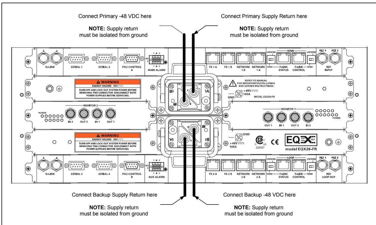
**Figure 2-6: Connecting the EQX to a -48VDC System**
