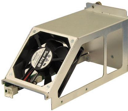
Each fan module is held in place by a single thumb screw and can be quickly and simply extracted and replaced from the front of the EQX frame should any one of them fail.
