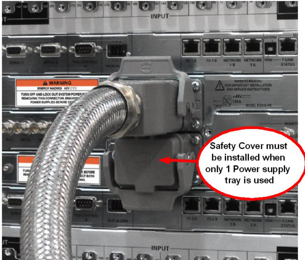
Figure 2-3: EQX External Power Supply – Connection to EQX
