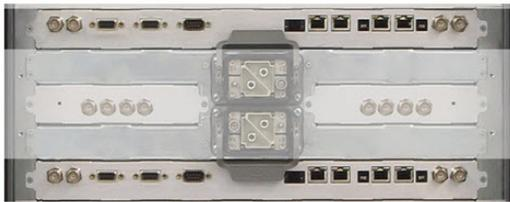
**Figure 5-3: F-LINK and Q-LINK Connectors**
