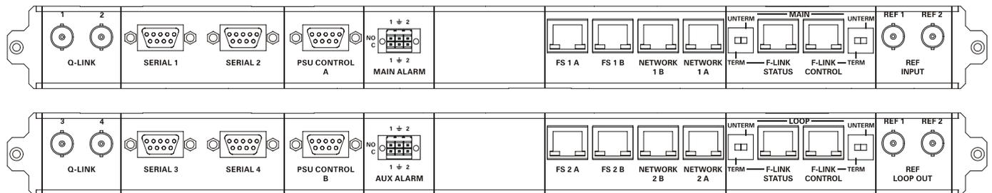
**Figure 5-4: EQX Communication Ports**
