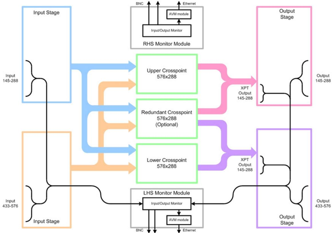
**Figure 5-9: EQX Signal Monitoring Path – Monitor 2 (LHS)**
