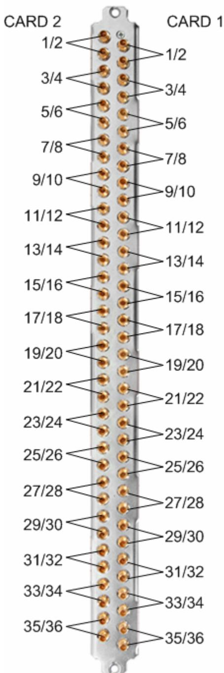
Figure 4-14: Double Density Output Fin
