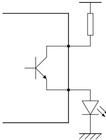
Figure 9-1: Example Alarm Circuit
