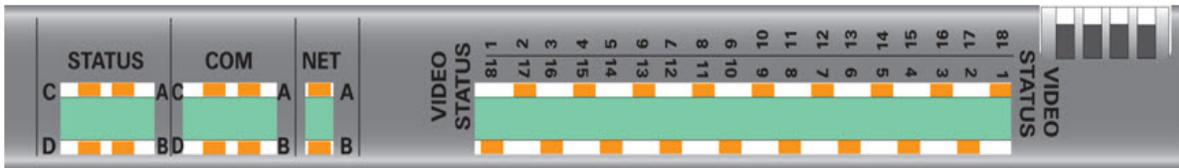
**Figure 4-6: Output Module – Air Dam Detail**
