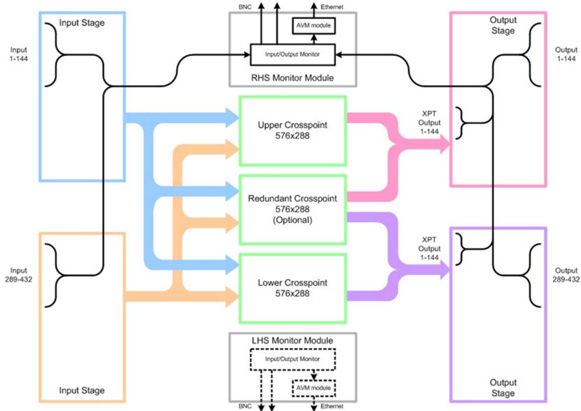
**Figure 5-8: EQX Signal Monitoring Path – Monitor 1 (RHS)**
