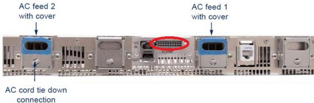
First, connect an Ethernet cable from the Control Network to the front of the PSU unit. Use a web browser to open the Power Supply Unit (PSU) web interface, login with username *Admin* and password *exadmin*. By default each PSU's IP is set to **192.168.0.230**.
