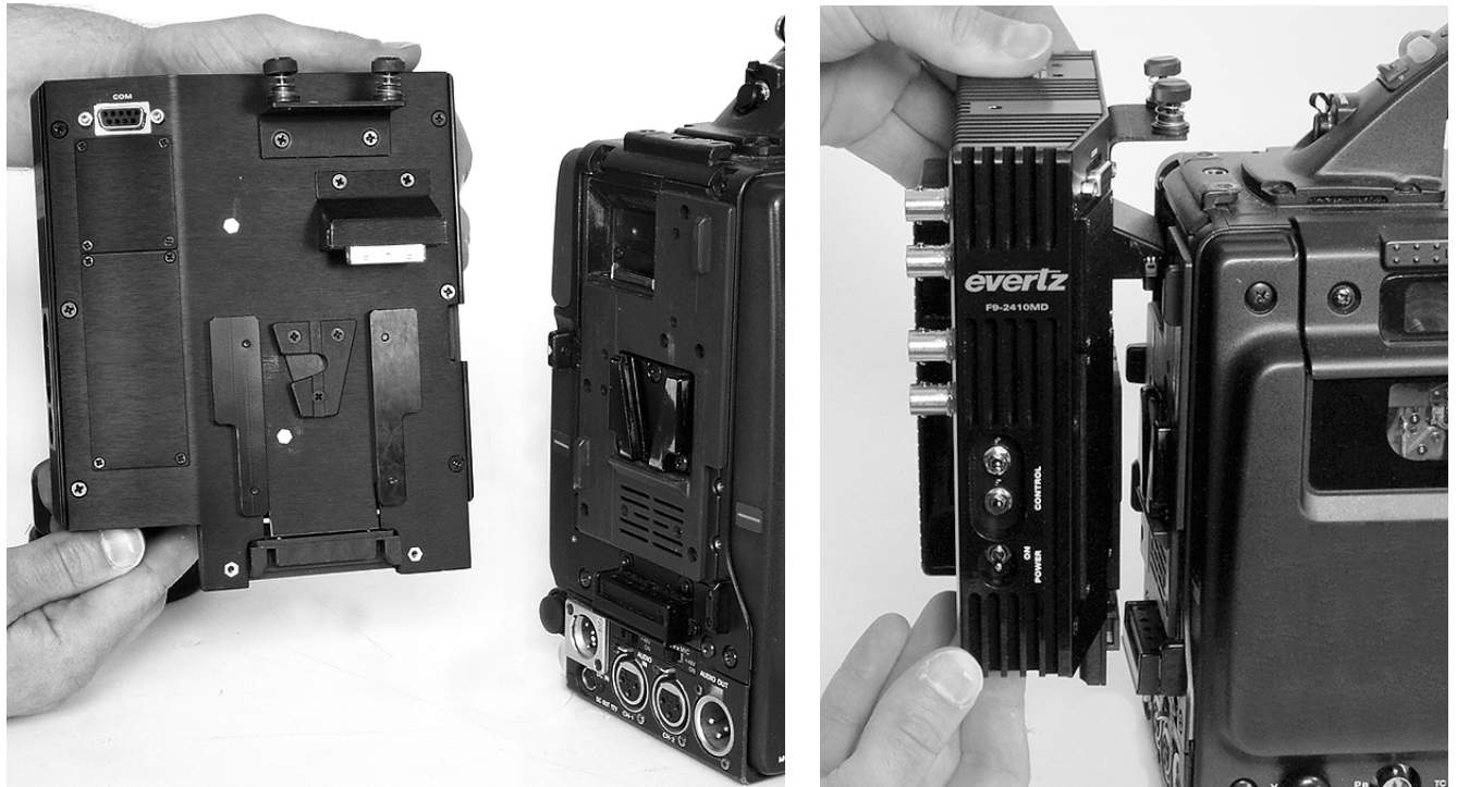
Figure 2: Mounting the F9-2410MD on the Rear of the Camera
