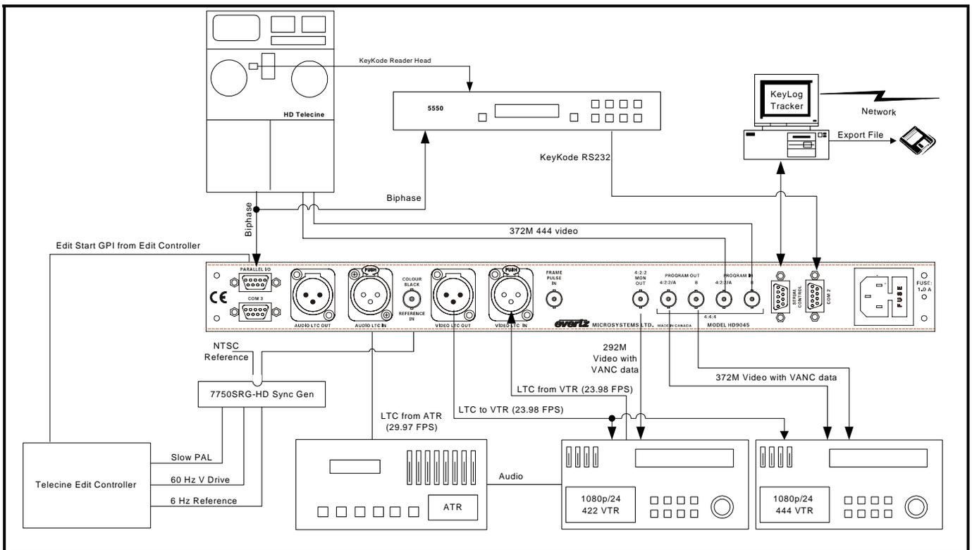
**Figure 2-2: High Definition (1080p/24) Connections**
