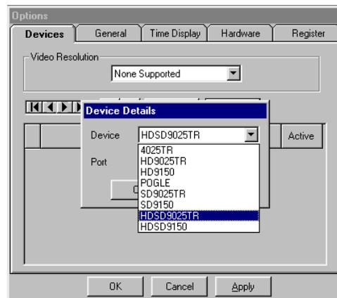
Click on the down arrow beside the *Port* dropdown and choose the COM port that you connected to the HD9045TR. Press the Okay button to add the HD9045TR to the list of controlled devices. If you need to
