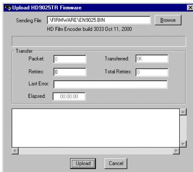
5. Use the BROWSE button to open the file dialog and choose the new firmware file. Typical filenames will be LP9045\_xxxx.BIN. (xxxx will be the build number of the software). The build version of the firmware will be shown in the dialog box.
