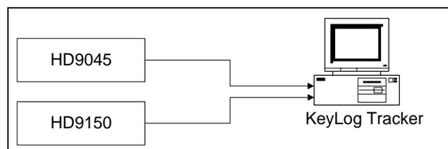
Figure 2-5: Connecting KeyLog Tracker to HD9045TR and HD9150Q using 2 COM Ports
