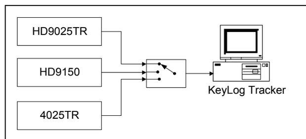
**Figure 4-3: Connecting KeyLog TRACKER™ to Multiple Devices Using A Single COM Port**
