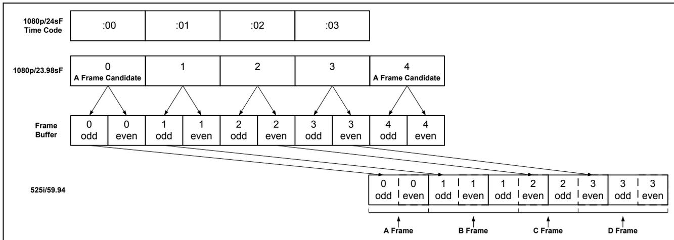
**Figure 5-1: Timecode Referenced 2:3 Pulldown and Delay in HD9155**
