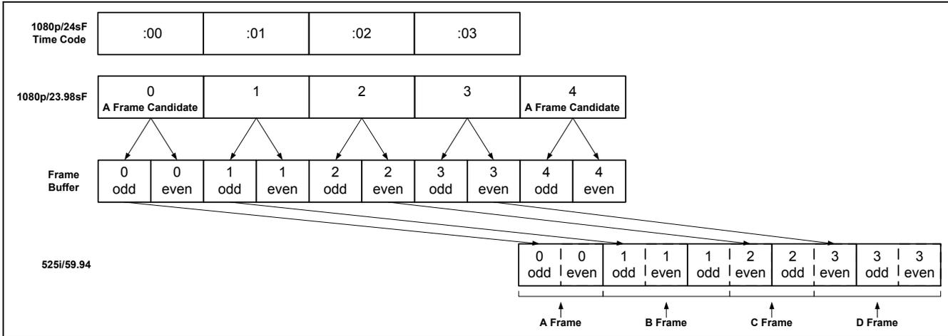
Figure 4-6: Timecode Referenced 2:3 Pulldown and Delay in HD9155
