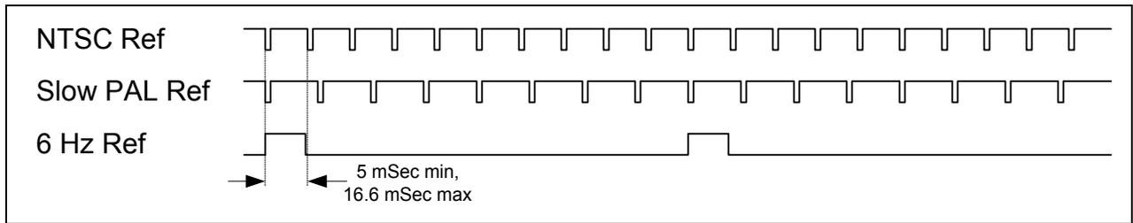
**Figure 4-4: 6 Hz Reference Pulse Timing**
