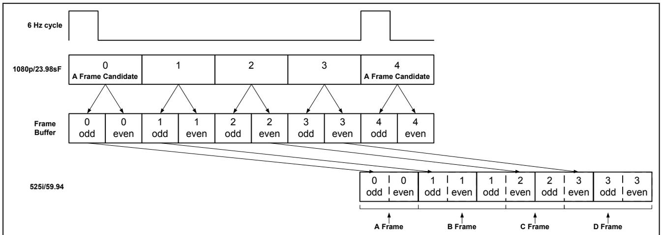
**Figure 4-5: 6 Hz Referenced 2:3 Pulldown and Delay in HD9155**
