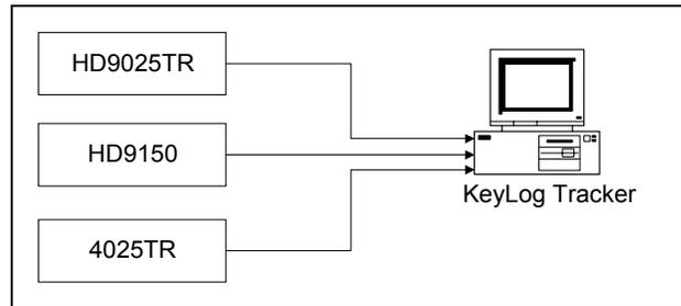
**Figure 4-2: Connecting KeyLog TRACKER™ to Multiple Devices using 3 COM Ports**
