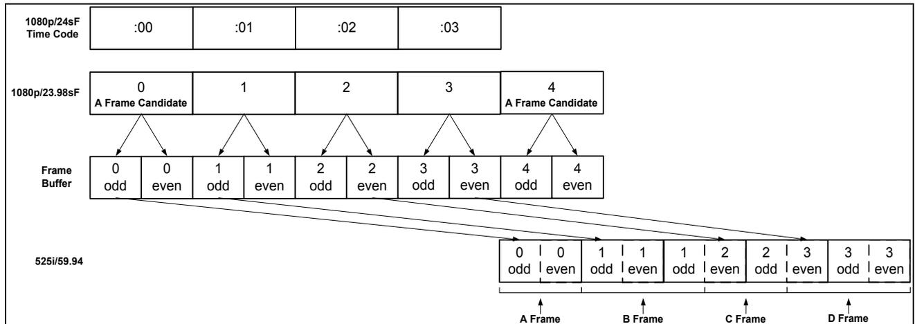
**Figure 3-5: Timecode Referenced 2:3 Pulldown and Delay in HD9155**
